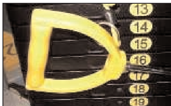
Right: A weight pin grip is large and open. The weight number labels are large, raised, and yellow (high contrast)
